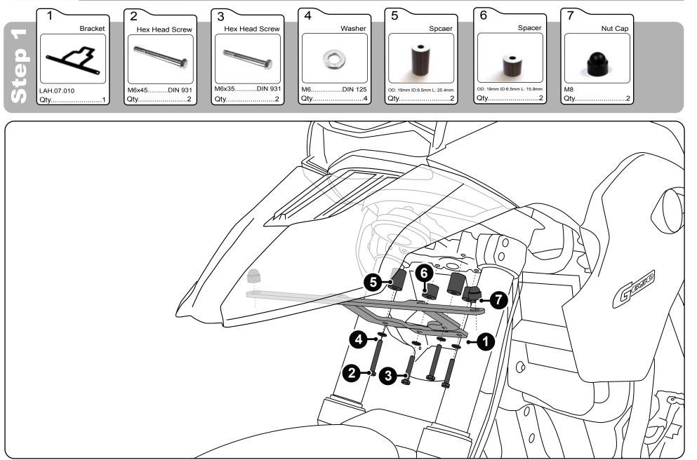
**Step One:** Remove the four bolts on the underside of the upper front fender. Use the supplied hardware to mount the light bracket to the motor-cycle, the longer bolts (#2) and spacers (#5) mount into the holes towards the front end of the motorcycle. Use the supplied Nut Caps (#7) to cover the nut used to mount the light pods to the bracket.
