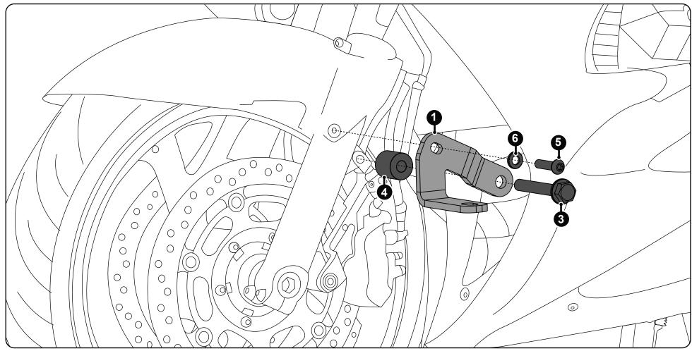
**Step One:** Remove the OEM fender bolt and OEM upper caliper bolt from the left side of the motorcycle. Use the bolts (#3 & #5), a washer (#6) and a spacer (#4) to bolt the left side bracket (#1) to the motorcycle. Repeat these steps on the right side of the motorcycle using the right side bracket (#2).
