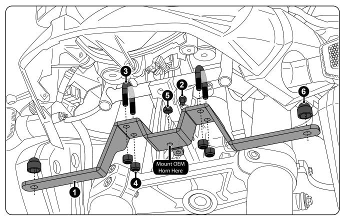
**Step One:** Take the rubber bumper (#2) and push it into the hole on the small tab on the rear of the mounting bracket (#1). Next take the OEM horn and bolt it to the center hole on the bracket (#1) using the supplied nut (#5).
