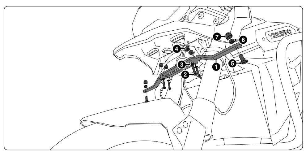
**Step One:** Remove the four OEM bolts on the underside of the upper front fender. Use a bolt (#2), a washer (#3) and a spacer (#4) to mount the light bracket (#1) to the four threaded holes. Hang the Light Pods downwards from the bracket using a bolt (#5), a nut (#6) and a nut cap (#7).
