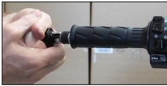
**TIPS:** To help with applying lubrication to the inside of the handlebar, loosen throttle housing and slide inwards. For left side use a screwdriver to lever grip end away from handlebar end. Be careful not to get lubrication between grip and outside of handlebar.
