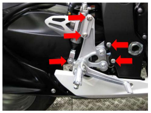
Having removed the original footrest, first connect the R&G Rear Set to the frame (1), but don't tighten it yet.
