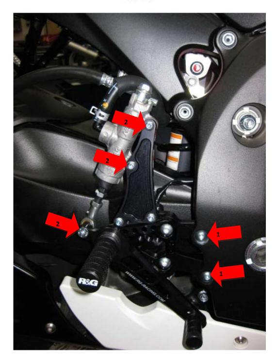
Then re-connect the rear brake master cylinder (2), find the right position and then tighten all screws.
