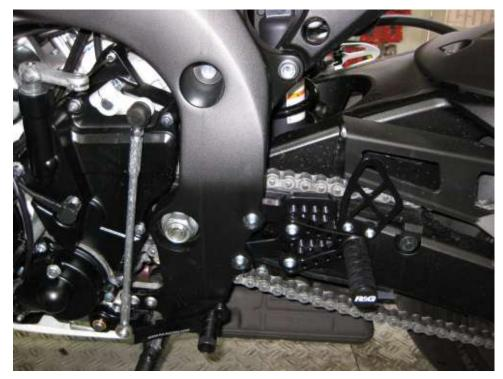
On the brake side, first remove the original footrest and disconnect the rear brake master cylinder.
