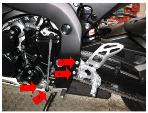
First remove the original gear lever (1), remove the lower connection (2) of the gear shaft and keep the original gear shaft on the bike. Then remove the original footrest.
