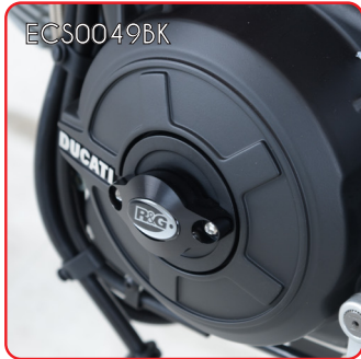
ENGINE CASE SLIDER
