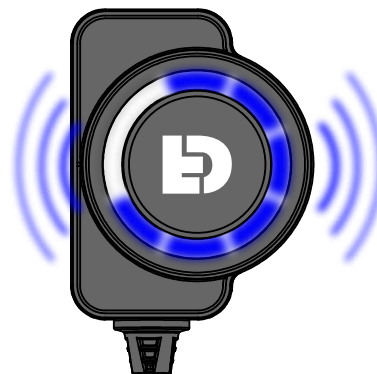
Flashing Blue LEDs Light Circuit One fuse setting mode
