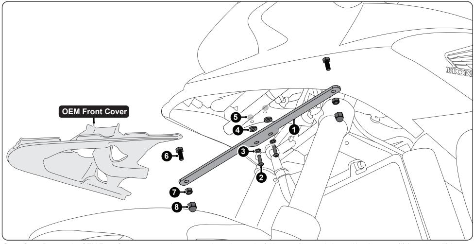
**Step One:** Remove the OEM Front Cover to expose the two mounting points on the fairing stay ilustrated above. Use the screw (#2), washers (#3), spacers (#4) and nuts (#5) to mount the bracket (#1) to the fiaring stay. Use the remaining hardware, bolts (#6), nuts (#7) and nut caps (#8) to mount the light pods to the bracket. They OEM Front Cover may be left off the bike, or can trimmed to reinstall over the bracket.
