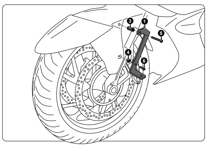
**Step One:** Remove the original fender bolts from the left hand side of the motorcycle. Next bolt the left hand side bracket in place using the supplied spacers and M6 hardware then torque each bolt to 7 ft-lbs.
