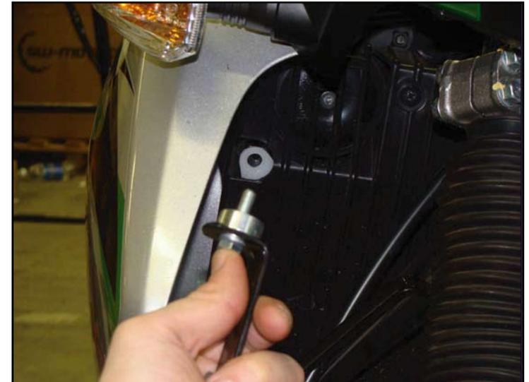
Attach the mounting bracket with the M6 screw provided. Place the 7mm spacer behind to the bracket.
