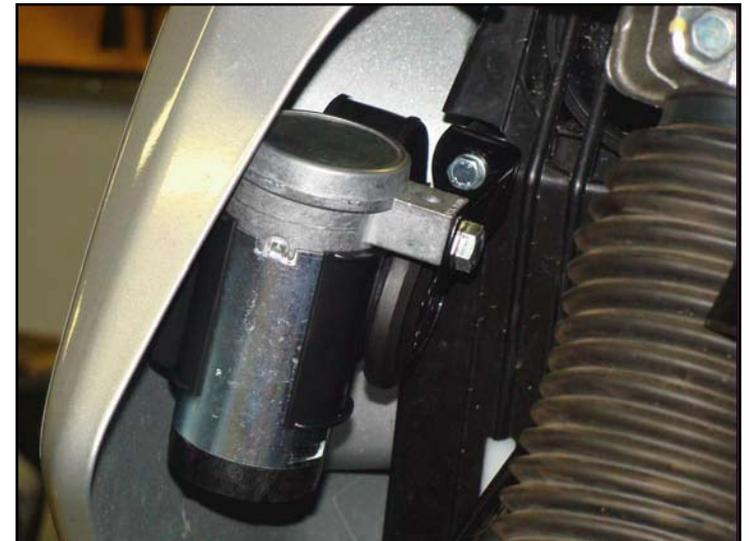
Mount the horn to the bracket using the hardware provided with the horn. Be sure to read all mounting instructions provided with the horn to ensure it is mounted at the right angle.
